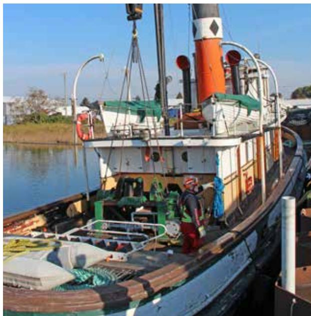
The steam-powered tow winch is chained up and ready to hoist.
